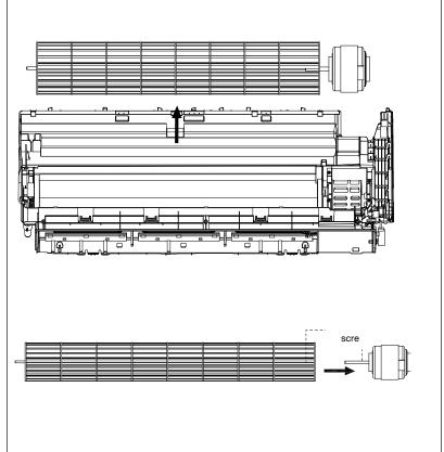
**ODU Disassembly Outdoor Unit Model Numbers:** YN009ALSI24RPG | YN012ALSI24RPG | YN009GLSI24RPG | YN012GLSI24RPG | YN018GLSI24RPG | YN024GLSI24RPG
