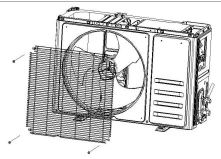
Unfix screws on front panel with fan guard, ODU middle separate plate and base plate, uplift front panel you can take it out from unit
