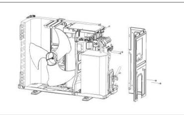
B Unfix the screws on the left plate, base plate, and condenser plate. Then take out the left plate.
