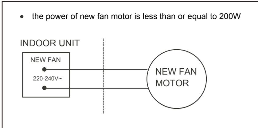
■ **Fig.10-10** (the figure is for the unit with the new fan function)
