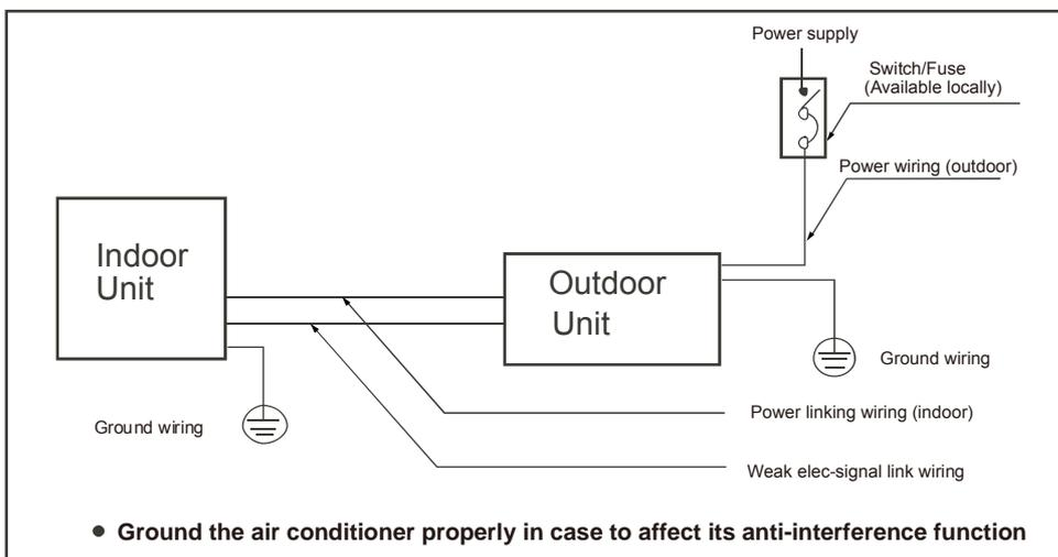
■ **Fig.10-9** (the figure is for the unit with the new fan function)
