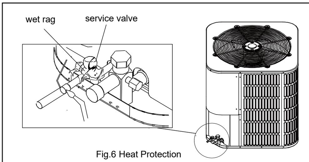
2. Braze the liquid line to the liquid valve at the outdoor unit. Be sure to wrap the valve body with a wet rag. Allow the nitrogen to continue flowing. Refer to the Tabular Data Sheet for proper liquid line sizing.
