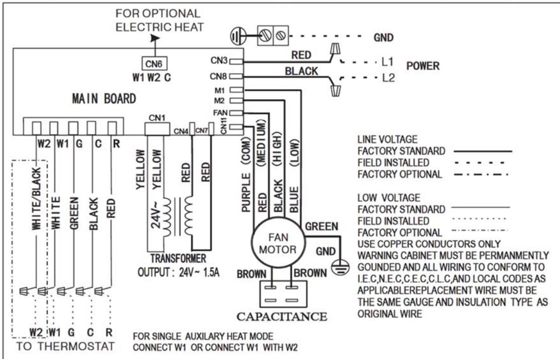
Indoor unit wiring diagram for ECM motor A/C systems and H/P systems (24K/36K/48K).
