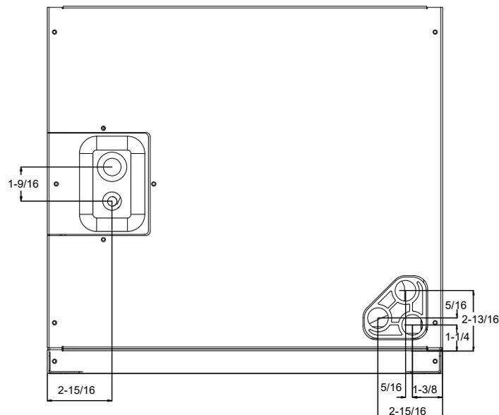
Fig.9 DIMENSIONS FOR FRONT CONNECT COIL
