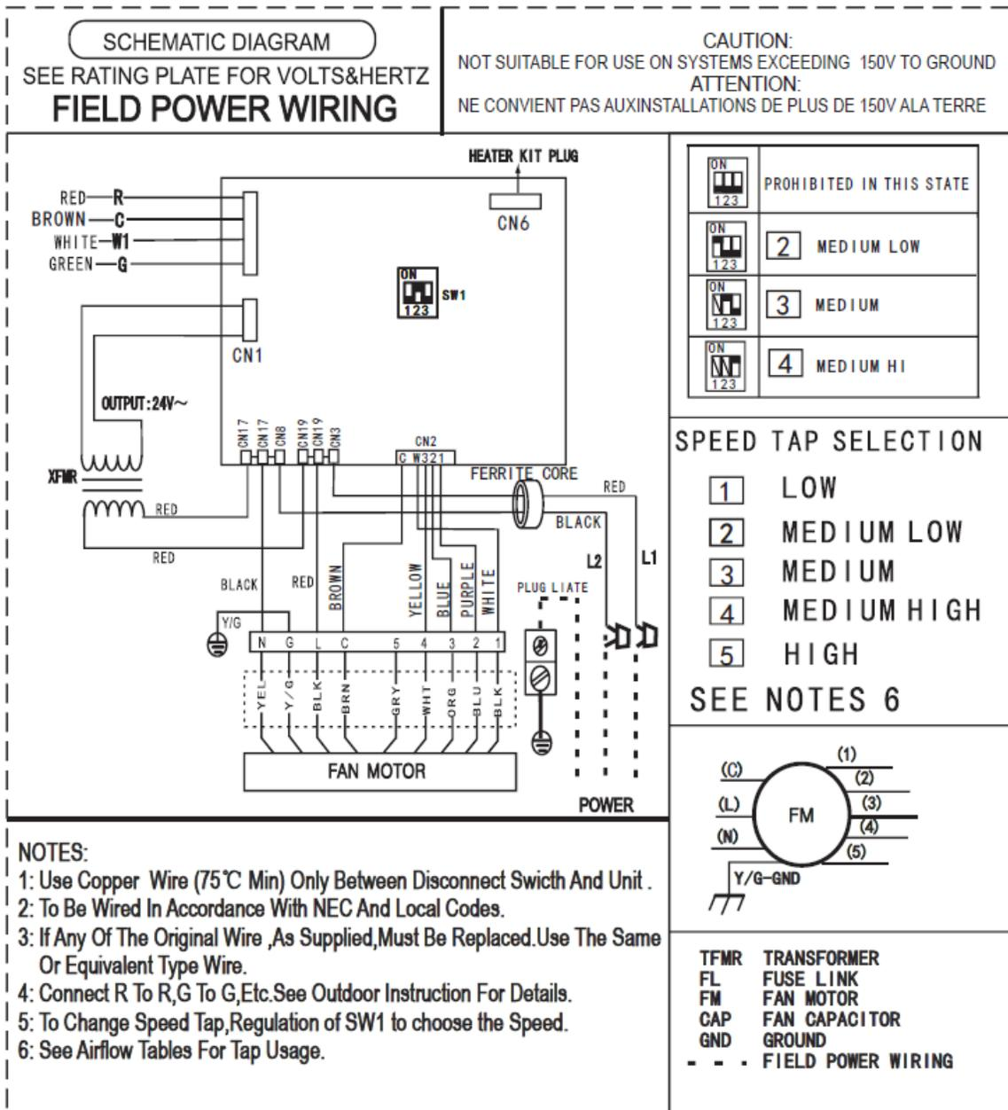
Indoor unit wiring diagram for ECM motor A/C systems and H/P systems (60K).
