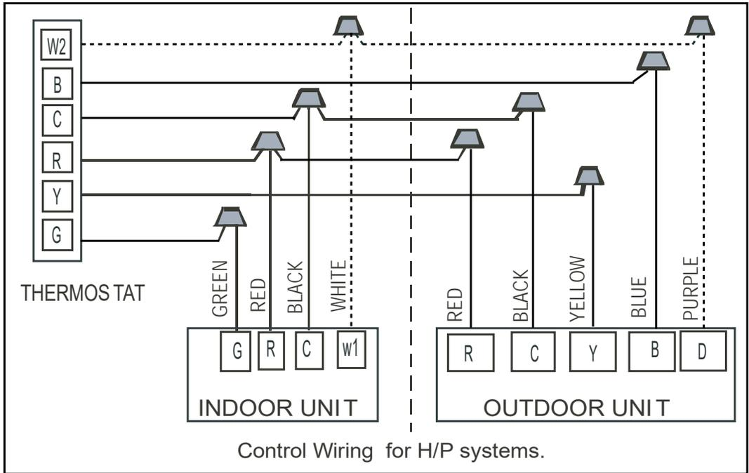
**Suggestion:** Thermostat choose KJR-25B or Non-programmed electrical thermostat series of Honeywell, such as TH 5220D. Broken lines means H/P system with electric heating. Wiring please refer to the Owner's Manual of the thermostat.
