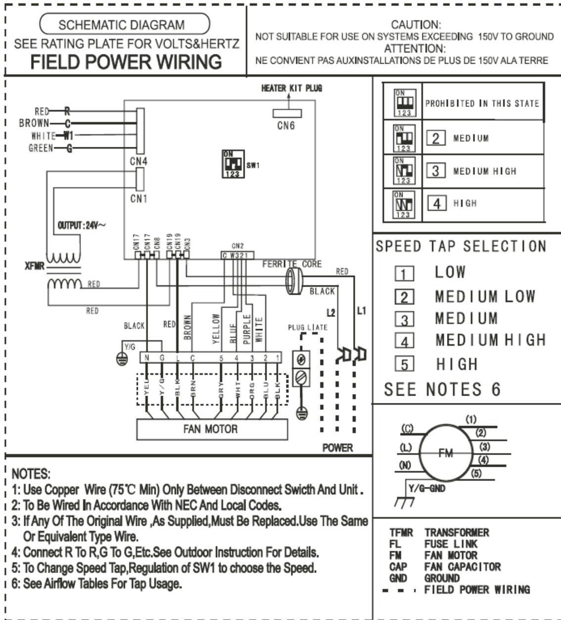
Indoor unit wiring diagram for electric heat.
