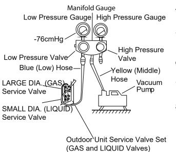
Connect the blue (low side) hose of the manifold gauge to the service port on the outdoor unit's GAS SIDE valve (use a 1/4" to 5/16" port adapter, if needed (sold separately))
