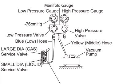
Outdoor Unit Service Valve Set (GAS and LIQUID Valves)
