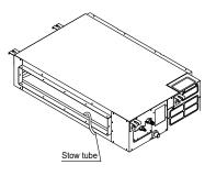
Fill the water pan with 2 liters of water. Check that the drainpipe is unhindered. Units WITH a Pump.
