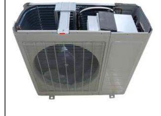
Fan ass'y How to remove the fan Electronic control box Fan ass'y. 1) After remove the panel plate following procedure 1, remove the hex nut fixing the fan and then remove the fan. Two reactors Compressor and liquid-gas separator Nut fixing the fan 2) Remove the one fixing screw. Unfix the hooks and then open the electronic control box cover.
