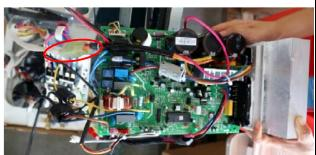
Remove the connector of electronic expansion valve.
