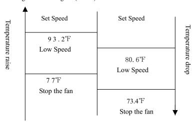
• During the heating operation, if the compressor stops that it will adjust the indoor fan speed, after 30 seconds to stop the fan.
