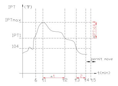
In the condition A, it must satisfy the conditions a), b)and c) then into defrosting operation.
