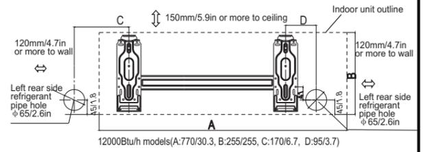
Correct orientation of Installation Plate
