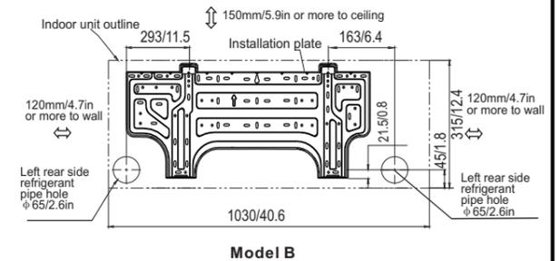
Correct orientation of Installation Plate
