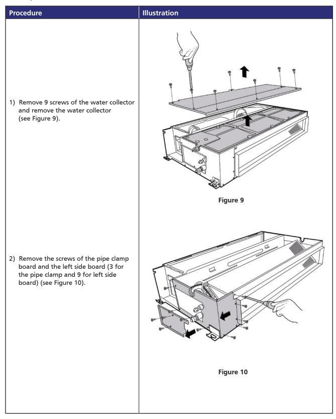
Note: Remove the front panel (refer to 1. Front panel) before disassembling electrical parts.
