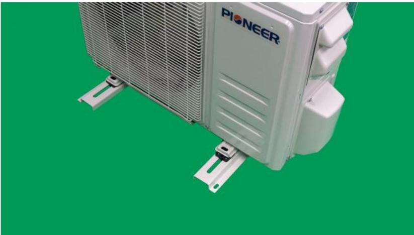
**Step 10: Use 4x M8-30 bolts+nut/washer to securely fasten the unit to the assembled bracket.**
