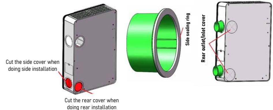
2. Since the above installation is for the "Side Installation Scenario", cut the EPS "Side Cover" located at the OA vent, as shown in the above picture. **DO NOT cut the EPS "Rear Cover" in this case.**
