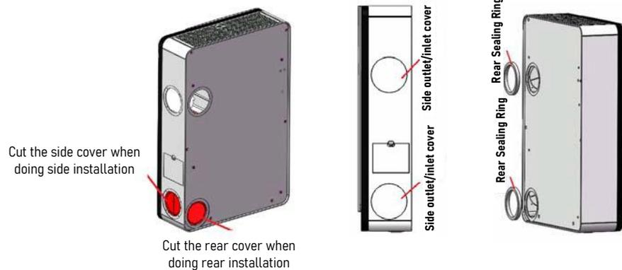
8. Place the 2 round OA and EA Side/Back covers on the side of the ventilator, to cover up the Side Air Inlet and Side Outlet (as shown above). Secure the 2x seal rings to the rear of the air inlet + outlet.
