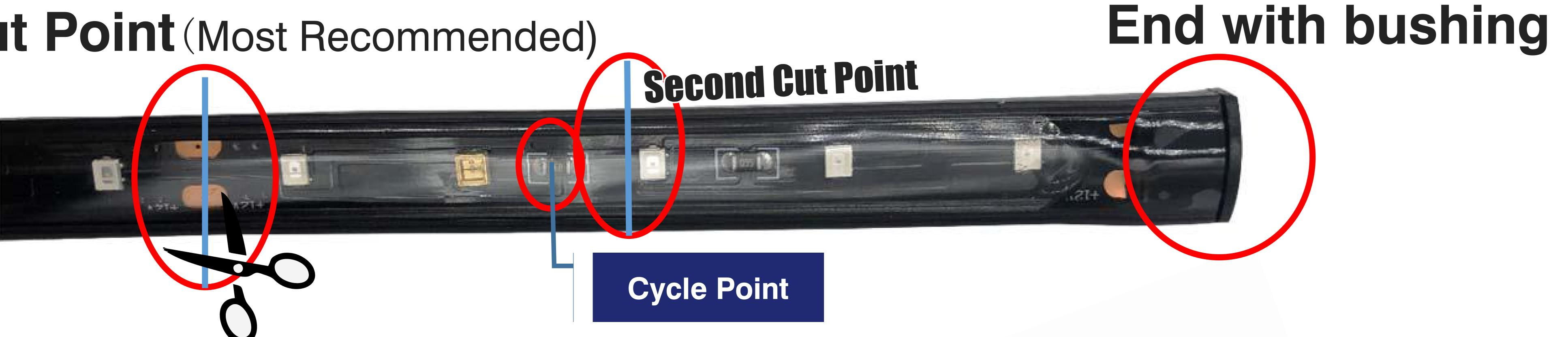
1. Determine how long you need to cut. 10 cm is a LED Modular Cycle.
