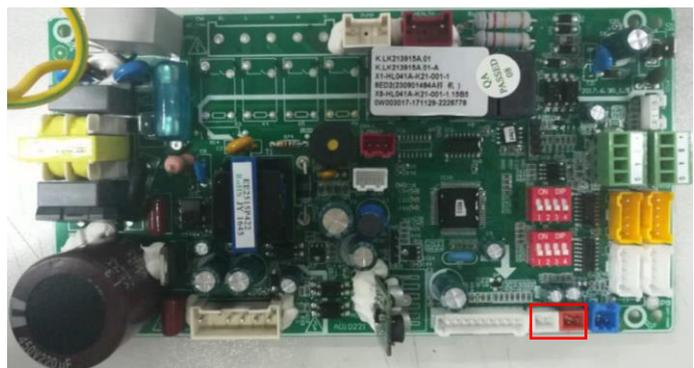
**Solution:** Check the connector of sensor and slot (CN6, CN6-1, CN6-2), if loose or not plugged in, please connect again.
