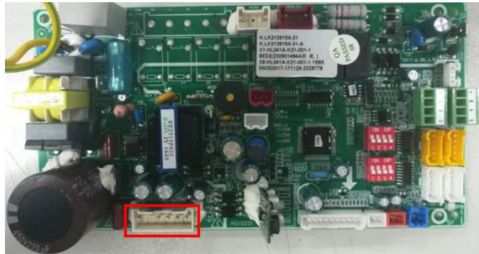
**Solution:** Check the connector of indoor motor and slot (CN3) and (CN4), if loose or not plugged in, please connect again.
