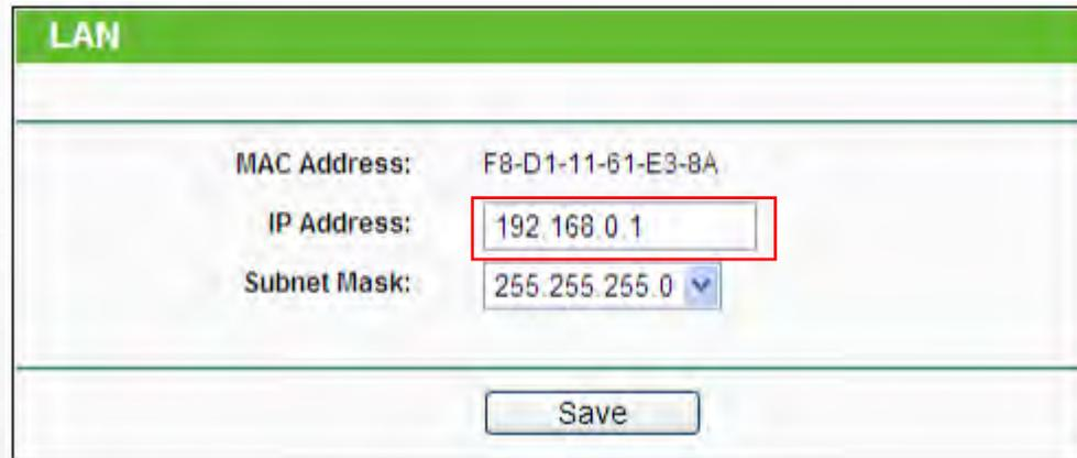
The screenshot shows a web-based configuration interface for a router's LAN settings. The title bar is green and labeled "LAN". Below it, there are three rows of configuration fields: "MAC Address" with the value "F8-D1-11-61-E3-8A", "IP Address" with the value "192.168.0.1" (highlighted by a red box), and "Subnet Mask" with a dropdown menu showing "255.255.255.0". At the bottom center, there is a "Save" button.
